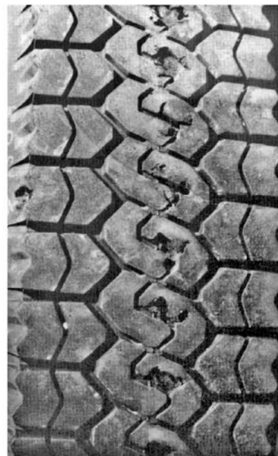
Example of Dyno Damage
