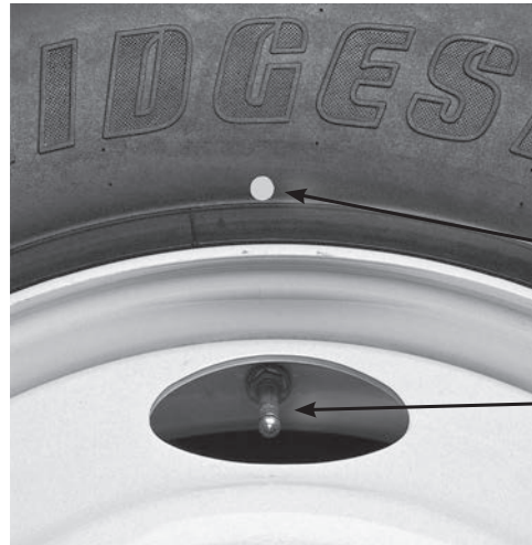
Tire light static balance mark (Yellow)
