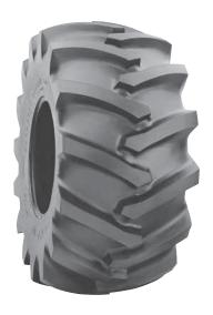
FLOTATION 23° DEEP TREAD (WTP) LOGGER - HF-4
