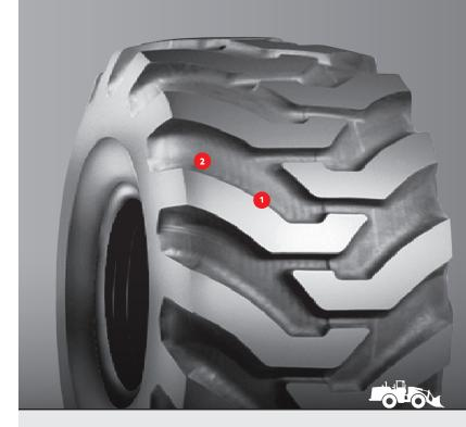
The Super Ground Grip Loader Dozer (SGG LD) bias ply tire features a self-cleaning directional tread designed for loader/dozer applications. Offers exceptional flotation and traction in soft soil or mud environments.
