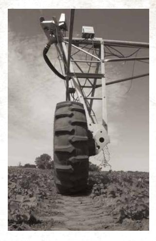
The tread design also helps to reduce soil disturbance and rutting conditions in the field.
