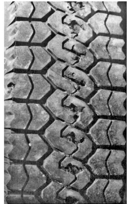
Example of Dyno Damage
