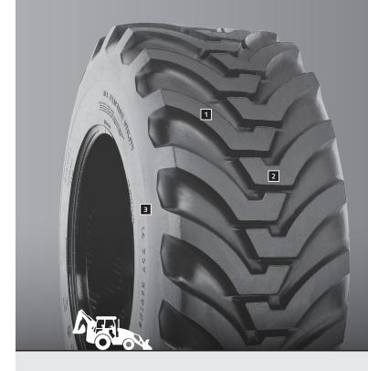
The All Traction Utility is designed specifically for light-construction machines such as loaders and backhoes, and is ideal for use on concrete and soil offering excellent traction and flotation.
