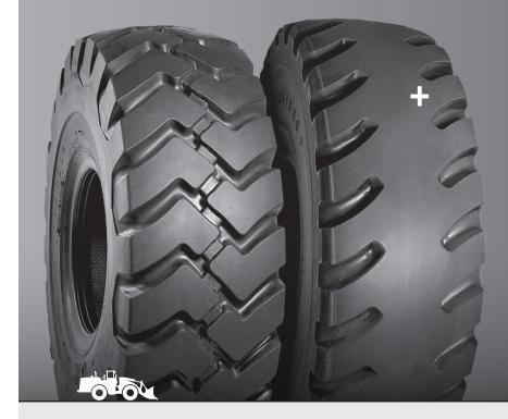
The Super Deep Tread Loader Dozer bias tire offers 250% deeper tread than L3 patterns providing greater casing protection and longer service life. Certain sizes available with "steel shield" construction for added cut and impact protection.
