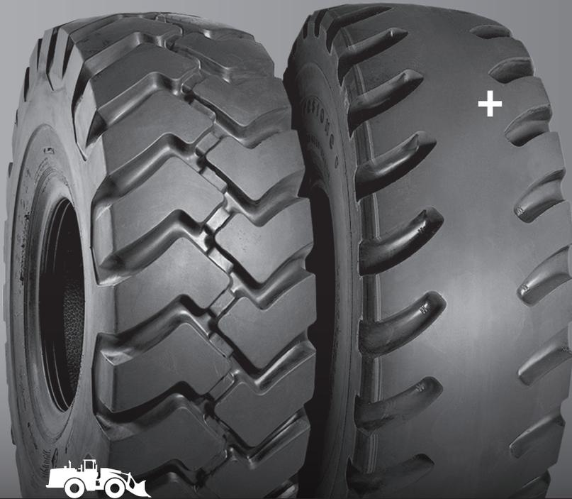
The Super Deep Tread Loader Dozer bias tire offers 250% deeper tread than L3 patterns providing greater casing protection and longer service life. Certain sizes available with "steel shield" construction for added cut and impact protection.
