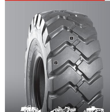
The Super Rock Grip™ bias tire offers a wide base for added stability and rubber compounds designed for wear resistance on improved surfaces in dock and in rail yard applications.
