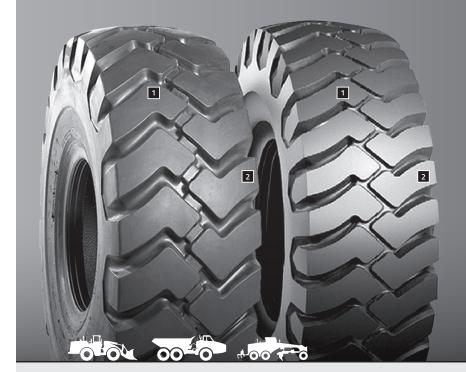
The Super Rock Grip™ Loader Dozer bias ply tire offers a heavy duty nondirectional tread design. It features exceptional traction and resistance to cutting and chipping in loader/dozer applications, as well as heat resistance in earthmover and grader service.
