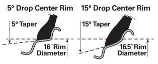
The following diagram shows how the beads of a 16" tire will not seat on a 16.5" rim. The beads cannot be forced out against the rim flanges by using more air pressure, because this will break the beads and the tire will explode.
