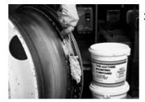
3. Lubricate the wheel bead seat using vegetable oil-based lubricant approved for both tire and wheel.
