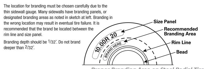
Proper Branding Area on Steel Radial Tire
