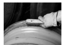
1. Remove dirt, rust or corrosion that can interfere with proper seal or damage bead.
