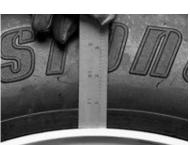
6. Measure distance from molded ring on tire to flange locations, 90 degrees apart.
