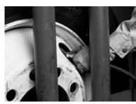
5. Inflate assembly to set bead and check for leaks around the wheel.
