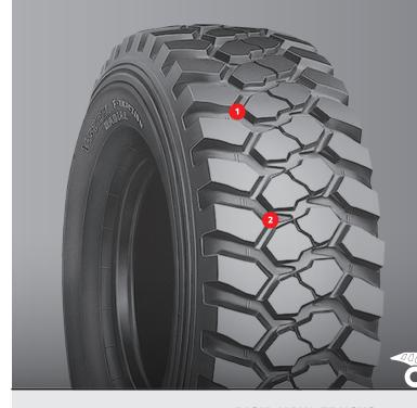
The V-Steel F-Traction (VFT) radial tire for haulage applications.
