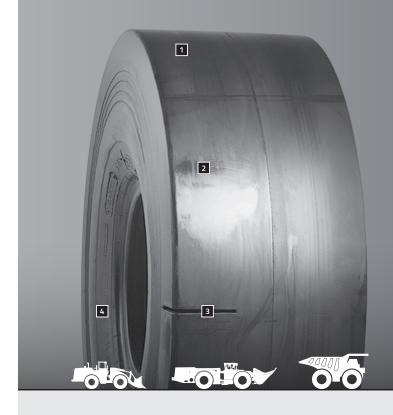
The Steel Smooth Tread Mine Service radial tire is ideal for underground mining, landfill, and salvage operations requiring maximum cut resistance and long tread wear contributing to lower operating costs.
