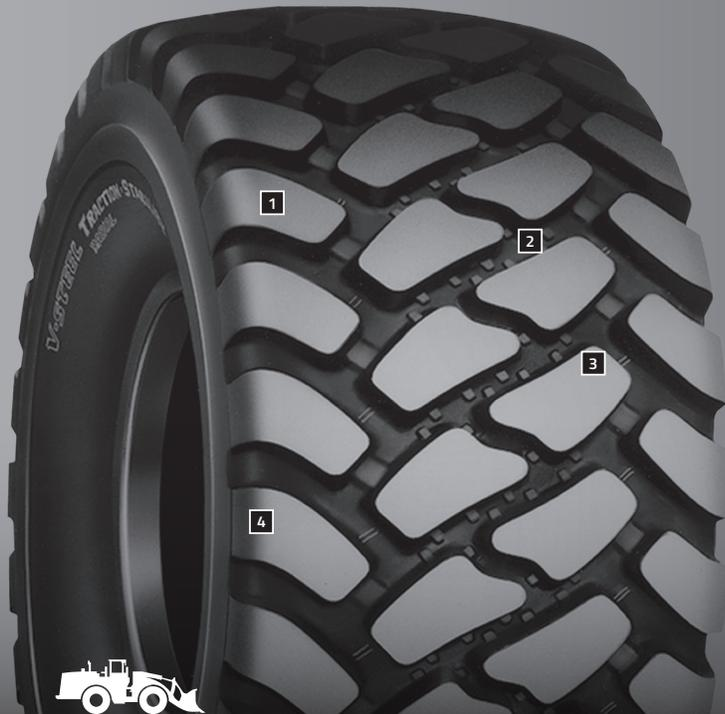
The V-Steel Traction and Stability radial tire features a low profile "65-series" design and provides excellent traction and improved stability in wheel loader applications.
